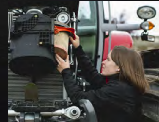
Engine air filter is easy to access and clean.
