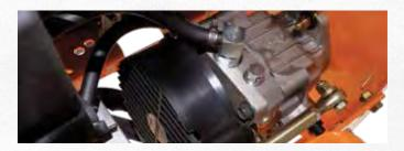
Dual 16 cc Hydro-Gear® pumps power this dependable drive system. Pump shock valves ensure reliability and long life. Cooling fans help maintain safe operating temperatures.
