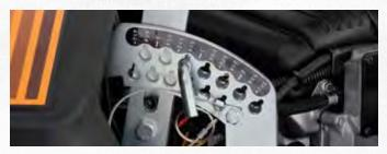
Easily change cutting heights in the field with no tools ( $1\frac{1}{2}$ " to  $4\frac{1}{2}$ " in  $\frac{1}{4}$ " increments). Deck can be lifted from the operating position with the pull of a spring-assisted lever.
