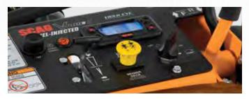
Easy-to-reach, full-featured instrument panel has ignition key, cutter-deck-engagement switch, throttle, choke and Tiger Eye Advanced Monitoring System. (Tiger Eye not available on 32" and 36" V-Ride II models.)
