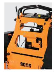
Comfort cushion and lower panel are removable to allow quick and easy service access to the hydraulic system.
