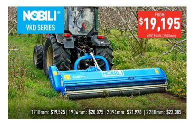
Designed for vineyard or orchard use where a finer mulch is produced from three mulching bars.
