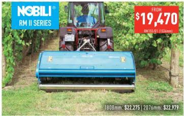
The Nobili RM II series mulchers are a robust and versatile machine with a helical blade pattern for a lower power requirement and life greased bearings.
