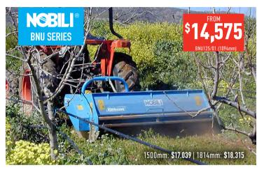
Multi-purpose machine suited to general clearing, pasture topping & vineyard prunings. Height control is maintained by adjustable skids.
